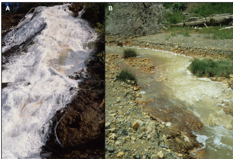
FIGURE 5.11 (a) White aluminous precipitate approximating the composition of basaluminite but amorphous to X-rays in effluent from a caved-in mine portal near Silverton, Colorado; (b) white aluminous precipitate in Leviathan Creek, near Markleeville, California
